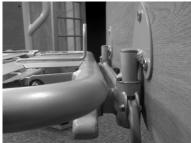
• When the assembly bar is pulled out to the first slot at the head of the bed and second slot at the foot of the bed it is at the 80" length.
